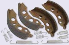
Al-ko type brake shoe kit 200mm x 50mm diameter. Kit contains four brake shoes and all springs required.
