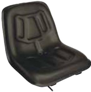
Black vinyl compact tractor seat with a universal mounting hole pattern and slide track with 170mm fore/aft travel. Height: 340mm, width: 380mm.
