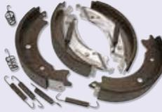
Knott type brake kit contains two fixed and two sliding brake shoes, auto-reverse sliding shoe carrier and all springs required. 203mm x 40mm diameter.
