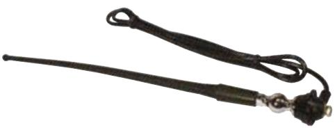
Universal wing or roof mount rubber aerial, single section rubber mast, fully extended length 405mm, coaxial screened connection cable and jack plug of 1270mm, adjustable angle head, robust vandal and damage resistant mast.
