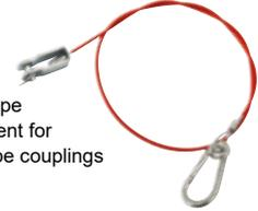
Clevis attachment for Knott type couplings
